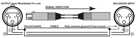
A great deal of mistakes in sound installations can be down to wrongly wired audio connections. It is important that the connections are correct to suit your system.
